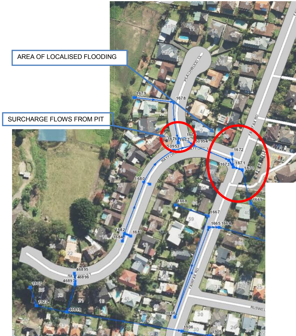
Figure 4 - Existing Network with Identified Issues
