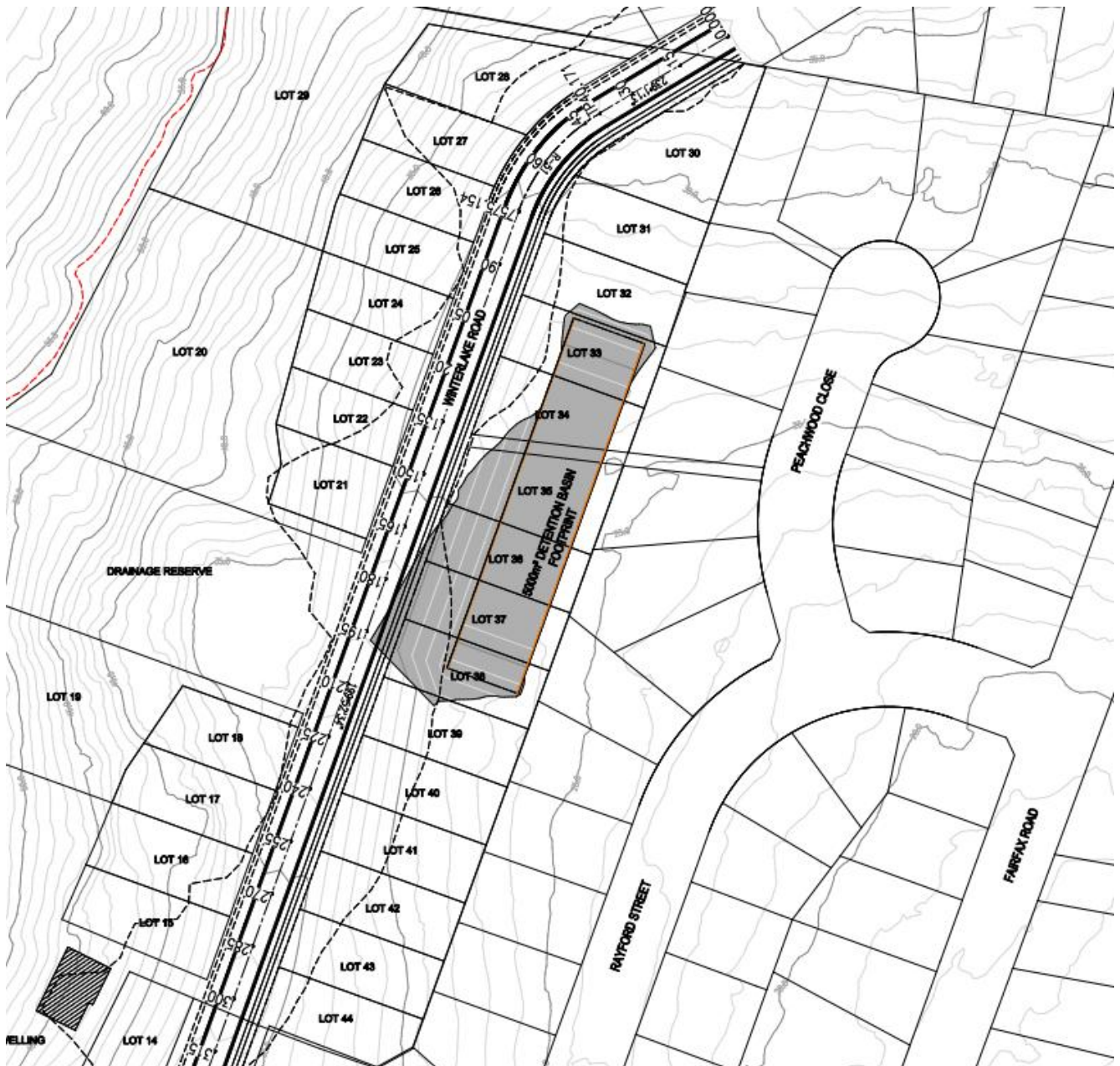
Figure 5 - Detention Basin Arrangement Option 1
