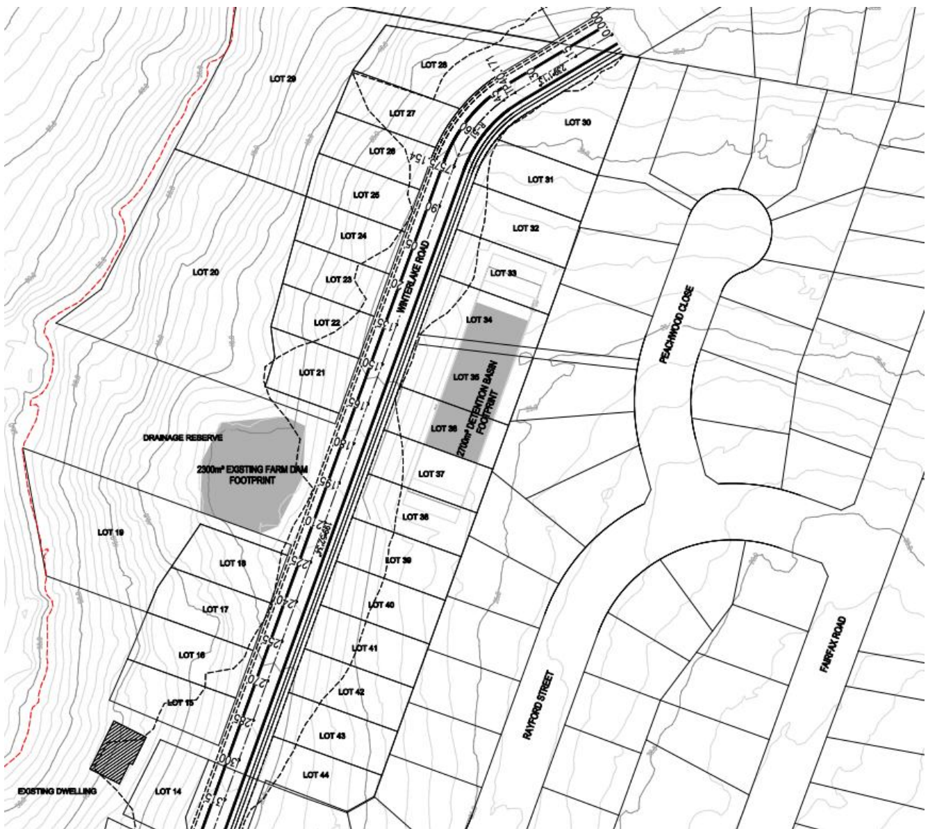
Figure 6 - Stormwater Detention Arrangement Option 2
